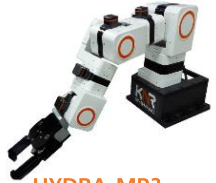
HYDRA-MP3 (KNR's Multi-Purpose Manipulator)
