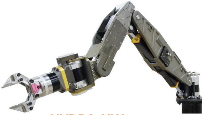
HYDRA-UW (KNR's Underwater Manipulator)
