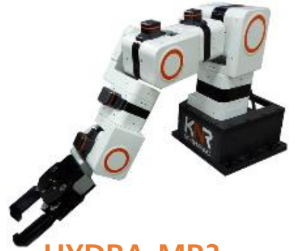
HYDRA-MP3 (KNR's Multi-Purpose Manipulator)
