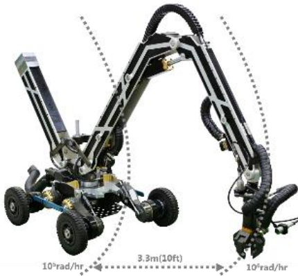
GIBBON (KNR's Hydraulic Mobile Robot in a nuclear power plant)
