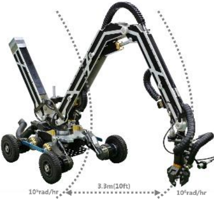
GIBBON (KNR's Hydraulic Mobile Robot in a nuclear power plant)
