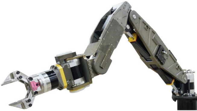
HYDRA-UW (KNR's Underwater Manipulator)
