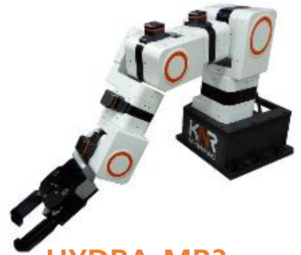
HYDRA-MP3 (KNR's Multi-Purpose Manipulator)
